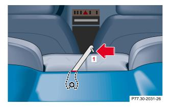
6. Place open-end wrench (1) (supplied in vehicle tool kit) on bolt between backrest and soft top compartment cover. Turn wrench (1) in direction of arrow to its stop and remove.
